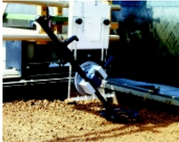
Guartel Detector during In-Soil Tests at TNO.
