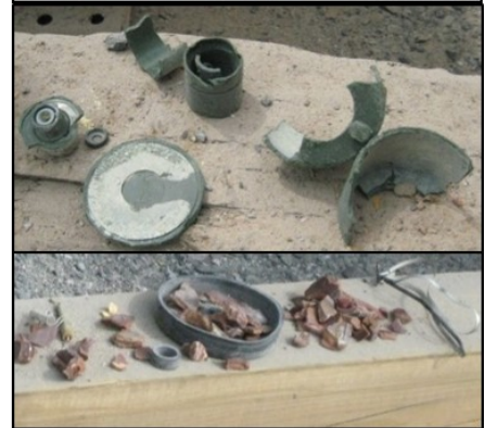
Live TAB-1 and PMN mines after crushing
