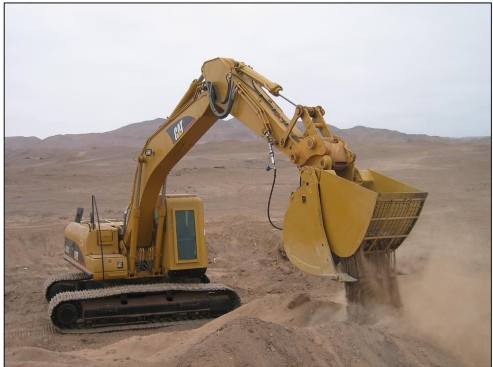
equipped with the right mix from the suite of more than a dozen tools, the system can be tailored to suit a variety of local conditions and requirements of the typical demining organizations.
