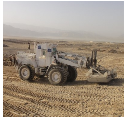
Magnet attachments reduce minefield clutter
