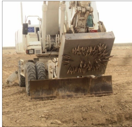
Magnet attachments reduce minefield clutter
