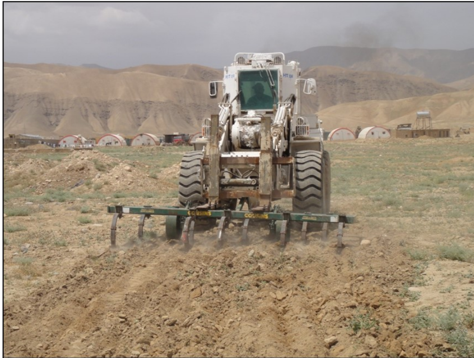
Mantis cultivator on HALO loader loosens soil for manual demining.
