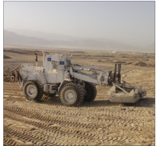
Magnet attachments reduce minefield clutter
