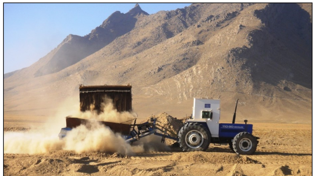
Modified Standen Pearson Megastar Soil Sifter
