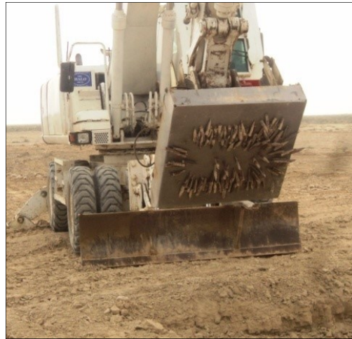
Magnet attachments reduce minefield clutter
