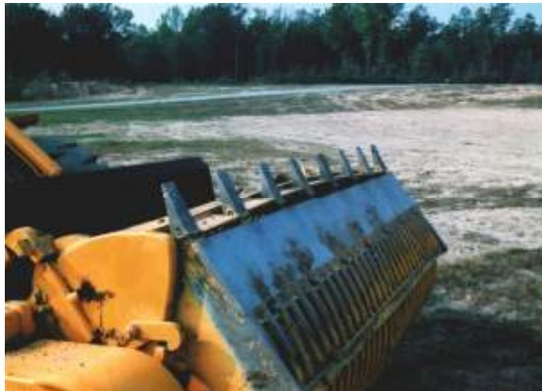
**Figure 16. Blast Distortion (Bowing) to ROTAR<sup>®</sup>**
