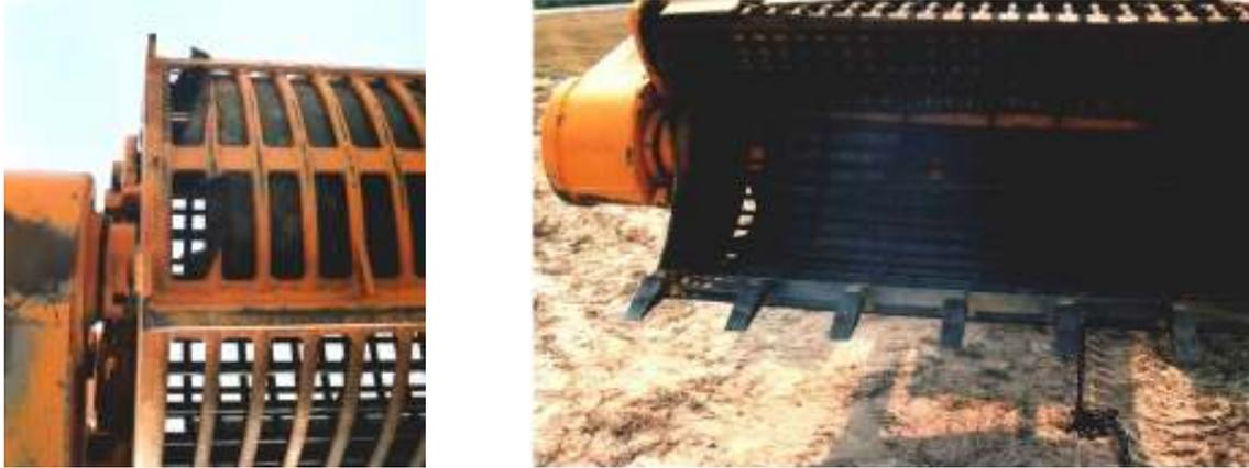
**Figure 17. Blast Test Damage to Steel Liner**
