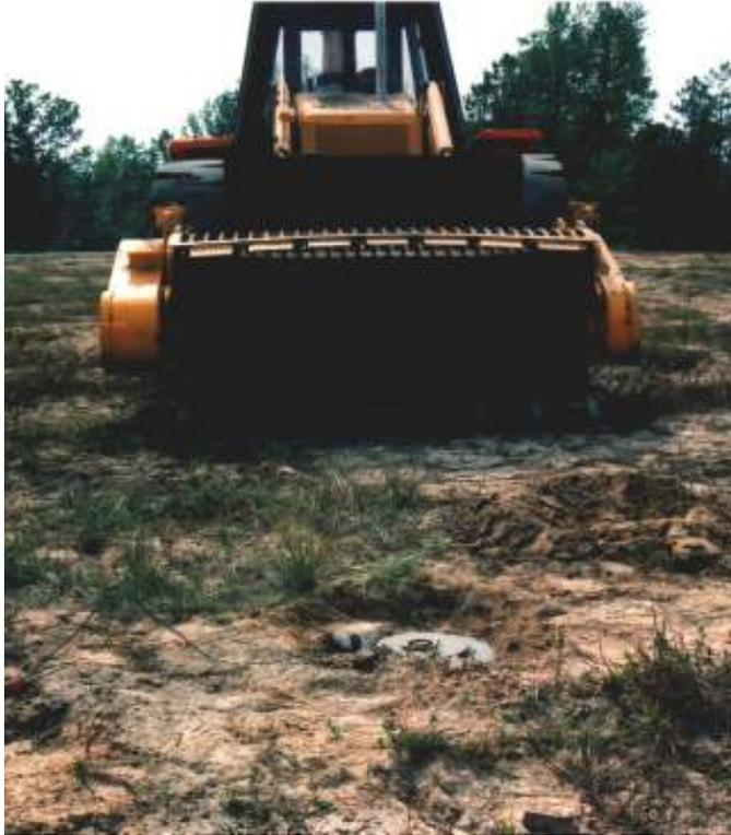
**Figure 20. Improved Backhoe Before AT Mine Detonation**
