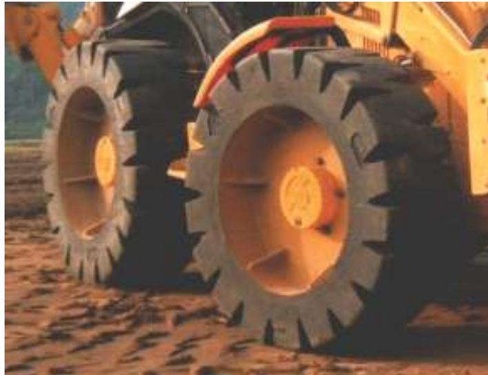
**Figure 4. SETCO Solid Rubber Tire**
