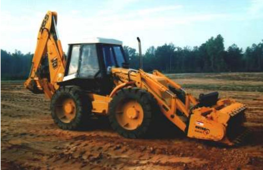
**Figure 1. Improved Backhoe With HPL 800 S ROTAR<sup>®</sup>**
