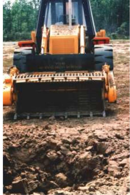
**Figure 21. Improved Backhoe After AT Mine Detonation**
